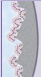
Section of pipe wall showing sharp points concentrating electrons which attract the ions for precipitation to surfaces.
